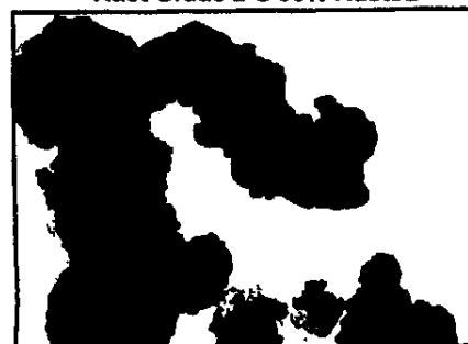
Rust Grade 1-S 50% Rusted
