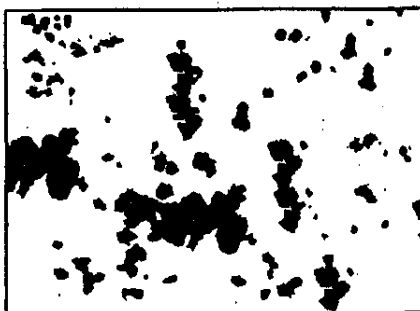
Rust Grade 3-G 16% Rusted
