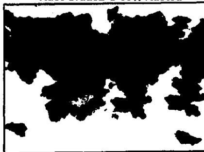
Rust Grade 1-G 50% Rusted
